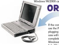
If the computer to be used is a notebook with a PCMCIA slot, use the PCM-WIN interface. Install the control software before plugging in the PCM-WIN interface card. The installation process will install the correct driver for the PCM-WIN card. After completing the installation, plug in the PCM-WIN card and Windows 95/98 should find the card and establish the correct link Windows NT will find the card on restart
